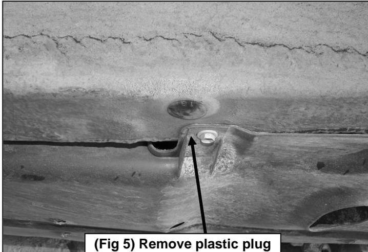
(Fig 5) Remove plastic plug on bottom of frame channel
